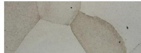
Heat treatment at 920°C-15 min + Quenching
